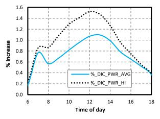
**FIGURE 4**: The diurnal pattern of differences in power output between the Dichondra test plot and the control (average for July 2020). Note the difference between values for the upper row of panels only (HI) and the average for the entire plot (AVG).
