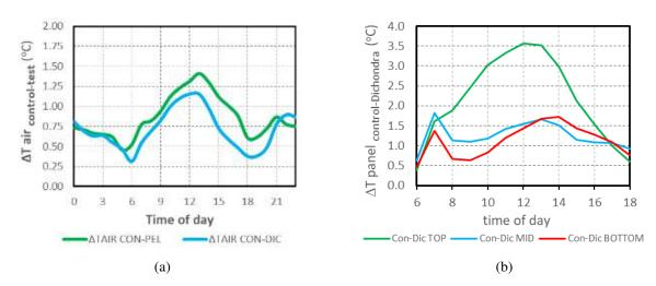
**FIGURE 3:** (a) difference in **air** temperature between control plot and test plots. (b) difference in **panel** temperature between control plot and test plots. In both figures, larger values indicate panels in test plots were cooler. Data for August 2020.
